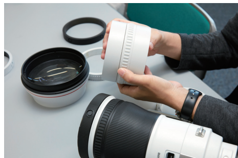
The knurled pattern and finger rests on the playback ring were studied to fine tune controls.
