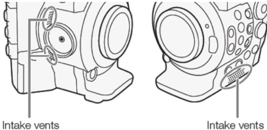
There are cooling holes on both the left and right sides of the camera body (fresh air intake), as well as at the top (warm air exhaust). *It is vital that these be open at all times, and not blocked with tape or covered by various accessories fitted to the camera.* Operators must be aware of the location of these cooling vents, and insure that the cooling system is not blocked in any way.
